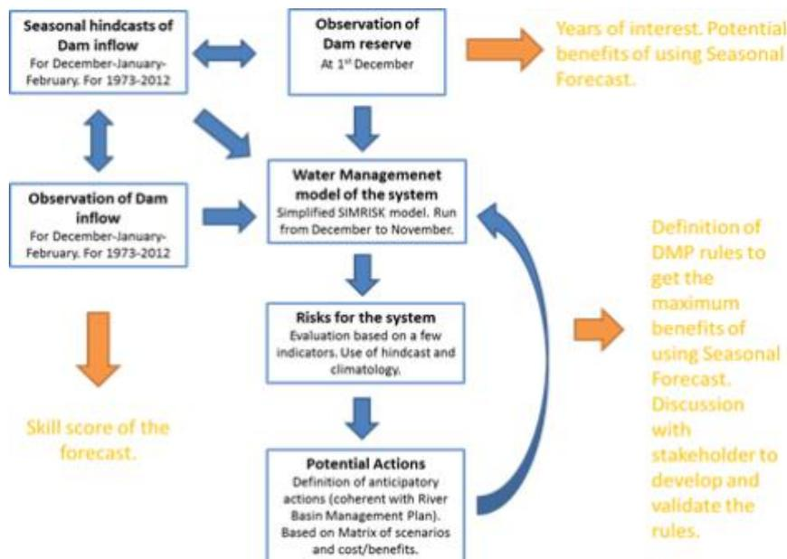
Figure 21 - General framework for the analysis of Decision Making Process Value for dam management in Spain
