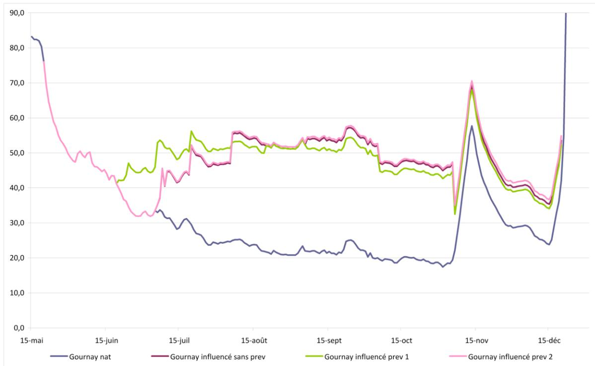
Figure 17 - Simulation of the river flows at the Gournay station for the year 1989 from the Placebo protocol
